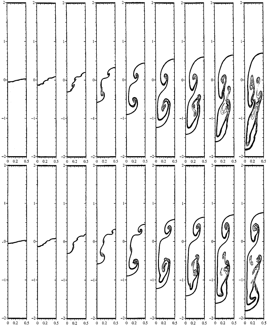
FIG. 5. Re = 1000 ; density ratio 7. The grid is composed of 30,189 \mathbb{P}_2 nodes (top) and 49,577 \mathbb{P}_2 nodes (bottom). The initial amplitude is 1% of the wavelength. The interface is shown at times 1, 1.5, 2, 2.5, 3, 3.5, 3.75, 4, and 4.25 (density contours 2 \leq \rho \leq 4 ).
